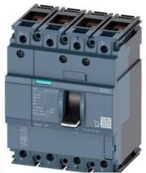
CIRCUIT BREAKER 3VA1 IEC FRAME 160 BREAKING CAPACITY CLASS H ICU=70KA @ 415 V 4-POLE, LINE PROTECTION TM210, FTFM, IN=32A OVERLOAD PROTECTION IR=32A FIXED SHORT CIRCUIT PROTECTION II=10 X IN NEUTRAL PROTECTION 100% BUSBAR CONNECTION
