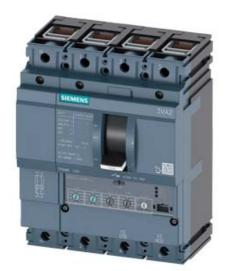
CIRCUIT BREAKER 3VA2 IEC FRAME 100 BREAKING CAPACITY CLASS C ICU=110KA @ 415 V 4POLE, LINE PROTECTION ETU350, LSI, IN=100A OVERLOAD PROTECTION IR=40A ...100A SHORT CIRCUIT PROTECTION ISD=1,5... 10 X IR, II=12 X IN NEUTRAL PROTECTION ADJUSTABLE(OFF,50%,100%) CABLE CONNECTION
