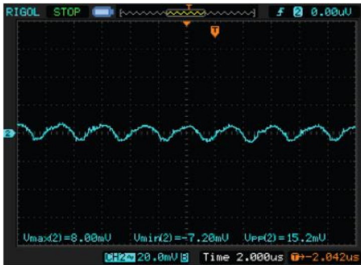
Figure 3. Output ripple at 2A load.
