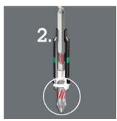
Higher peak loads are minimised through the torsion effect of the bit shaft (Phase 2). This effect is achieved with a specific heat treatment after the hardening process of the bits. This reduces the hardness of the shaft in comparison to the drive tip.
