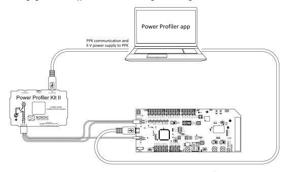
Figure 6: Measuring current in Ampere Meter mode
