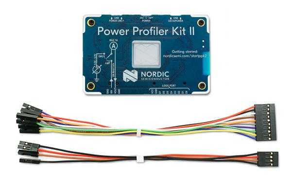
Figure 1: PPK2 board and cables
