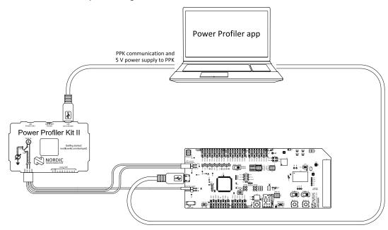
Figure 2: Typical configuration for measuring current on the DK
