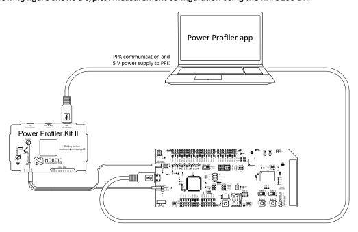
Figure 5: Measuring current in Source Meter mode
