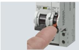
• Fault signal contacts with TEST and RESET button enable the simple testing of auxiliary circuits and, in the event of a fault, acknowledgement of the fault over the RESET button, without the need to switch the miniature circuit breakers.
