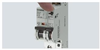
The auxiliary switches with TEST button enable the simple manual testing of control circuits during operation of the entire plant without the need to switch the miniature circuit breakers.
