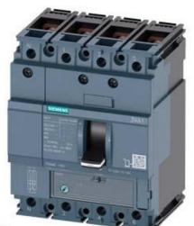
CIRCUIT BREAKER 3VA1 IEC FRAME 160 BREAKING CAPACITY CLASS N ICU=25KA @ 415 V 4-POLE, LINE PROTECTION TM220, ATFM, IN=160A OVERLOAD PROTECTION IR=112A ...160A SHORT CIRCUIT PROTECTION II=10 X IN NEUTRAL UNPROTECTED BUSBAR CONNECTION
