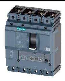
CIRCUIT BREAKER 3VA2 IEC FRAME 250 BREAKING CAPACITY CLASS H ICU=85KA @ 415 V 4POLE, LINE PROTECTION ETU330, LIG, IN=160A OVERLOAD PROTECTION IR=64A ...160A SHORT CIRCUIT PROTECTION II=1,5...12 X IN NEUTRAL PROTECTION ADJUSTABLE(OFF,50%,100%) GROUNDFAULTPROTECTION IG=0,2... 1 X IN, TG=0,1/0,3MS BUSBAR CONNECTION
