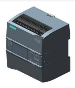
SIMATIC S7-1200, CPU 1212C, COMPACT CPU, AC/DC/RLY, ONBOARD I/O: 8 DI 24V DC; 6 DO RELAY 2A; 2 AI 0 - 10V DC, POWER SUPPLY: AC 85 - 264 V AC AT 47 - 63 HZ, PROGRAM/DATA MEMORY: 75 KB
