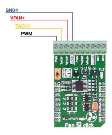
A single onboard jumper setting enables 2 or 3 wire fan connection. In addition, there are two points (DXP, DXN) on the same terminal for external temperature sensor connection. The click communicates with the MCU over data interface voltage level of 3.3V only.
