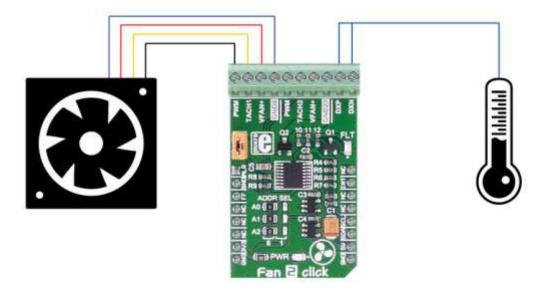
For example, you can set the limit at 25°C and if the temperature goes over that the click will activate the fan; it will keep working until the temperature is 25°C again.
