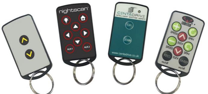
**Changing the Battery:** Remove the enclosure screws. Replace Coin Cell battery (CR2032), taking care of contacts and the battery polarity
