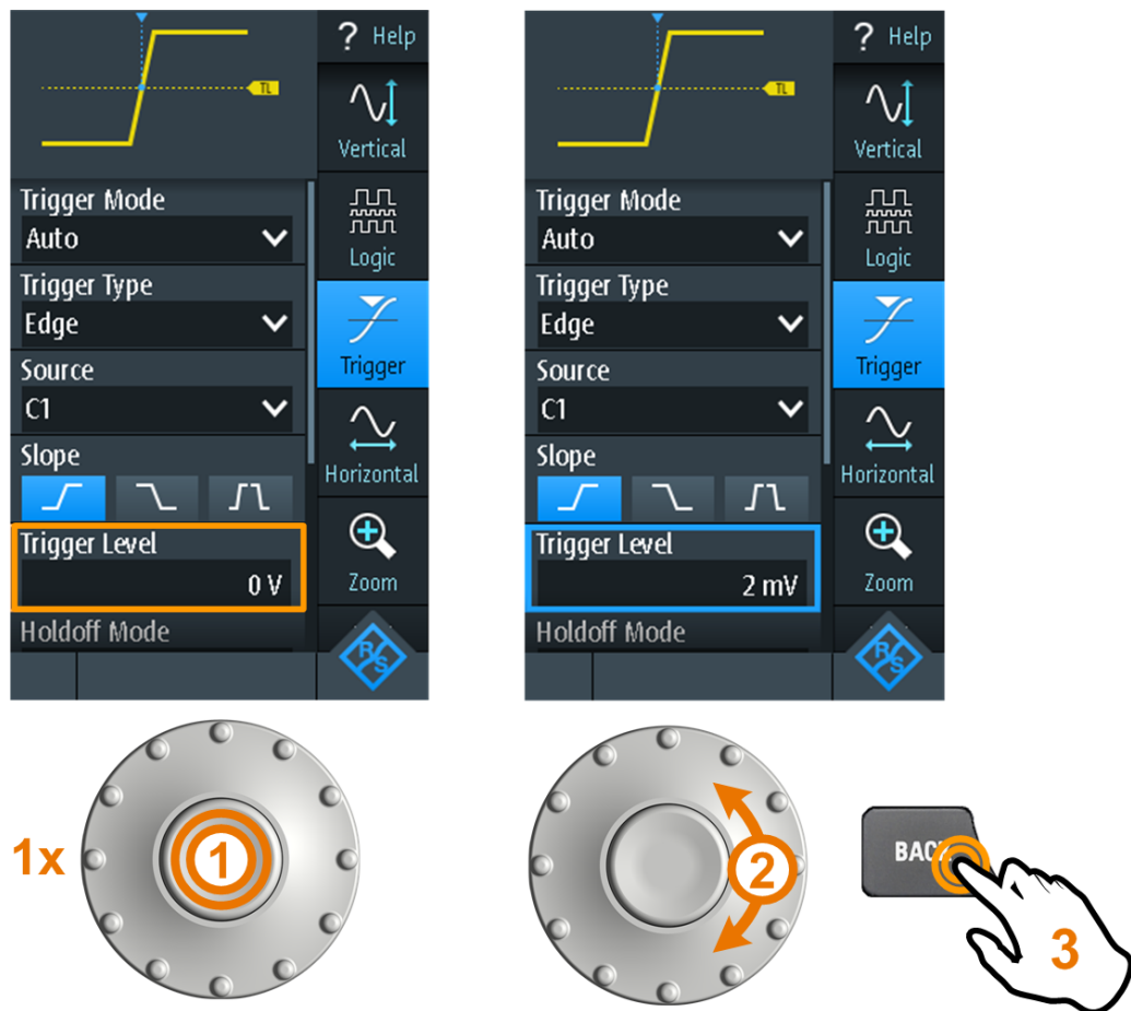
Figure 1-11: Set numerical value using the wheel
