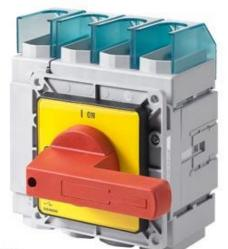
MAIN SWITCH 4-POLE FRONT MOUNTING IU=160A, P/AC-23A AT 400V=75KW ROTARY ACTUATOR RED/YELLOW (EMERG. STOP) FOUR-HOLE MOUNTING
