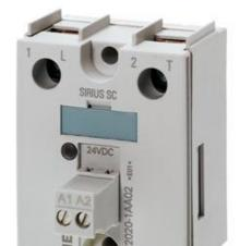
SEMICONDUCTOR RELAY 3RF2, 1-PH. WIDTH 45 MM, 20 A 24-230 V / 110-230 V AC SCREW TERMINAL
