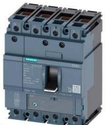
CIRCUIT BREAKER 3VA1 IEC FRAME 160 BREAKING CAPACITY CLASS N ICU=25KA @ 415 V 4-POLE, LINE PROTECTION TM220, ATFM, IN=160A OVERLOAD PROTECTION IR=112A ...160A SHORT CIRCUIT PROTECTION II=10 X IN NEUTRAL PROTECTION 50% CABLE CONNECTION
