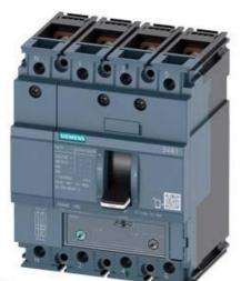
CIRCUIT BREAKER 3VA1 IEC FRAME 160 BREAKING CAPACITY CLASS S ICU=36KA @ 415 V 4-POLE, LINE PROTECTION TM240, ATAM, IN=63A OVERLOAD PROTECTION IR=44,1A ...63A SHORT CIRCUIT PROTECTION II=5...10 X IN NEUTRAL UNPROTECTED BUSBAR CONNECTION
