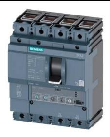
CIRCUIT BREAKER 3VA2 IEC FRAME 160 BREAKING CAPACITY CLASS L ICU=150KA @ 415 V 4POLE, LINE PROTECTION ETU350, LSI, IN=25A OVERLOAD PROTECTION IR=10A ...25A SHORT CIRCUIT PROTECTION ISD=1,5... 10 X IR, II=12 X IN NEUTRAL PROTECTION ADJUSTABLE(OFF,100%) CABLE CONNECTION
