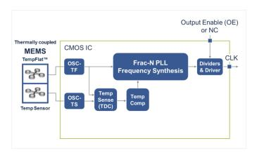
Figure 20. Block Diagram - TCXO
