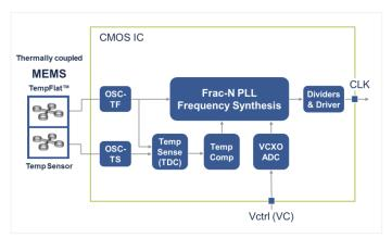
Figure 22. Block Diagram - VCTCXO
