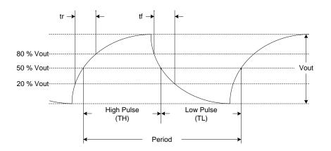
Figure 15. Clipped Sinewave Waveform Diagram
