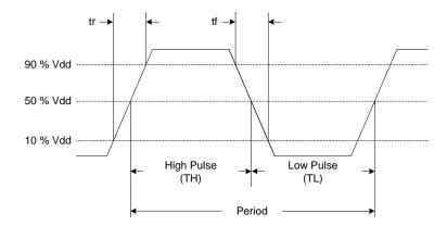
Figure 14. LVCMOS Waveform Diagram
