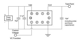
Figure 8. LVCMOS Test Circuit (VC Function)
