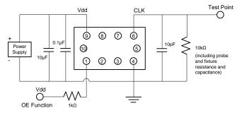
Figure 6. LVCMOS Test Circuit (OE Function)
