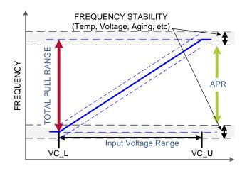
Figure 26. Typical SiTime VCTCXO FV Characteristic
