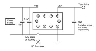
Figure 10. LVCMOS Test Circuit (NC Function)
