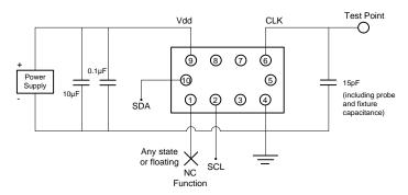
Figure 12. LVCMOS Test Circuit (I<sup>2</sup>C Control)
