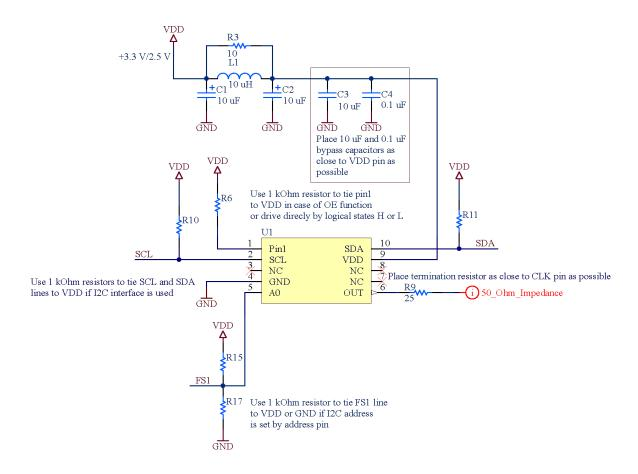
Figure 36. Schematic Example - DCTCXO
