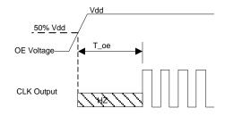
T\_oe: Time to re-enable the clock output
