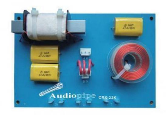
Speaker Crossover Network Perfect for new speaker designs, repair or upgrade. All input and output connections accept 1/4'' quick-disconnects, or may be soldered (recommended). Selectable 4ohm or  $8\Omega$  impedance, 12dB per octave, 2KHz crossover point. Maximum power capacity is 600W.
