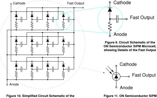
ON Semiconductor SiPM showing only a 12 Microcell Example. Typically, SiPM Sensors have Hundreds or **Thousands of Microcells**
