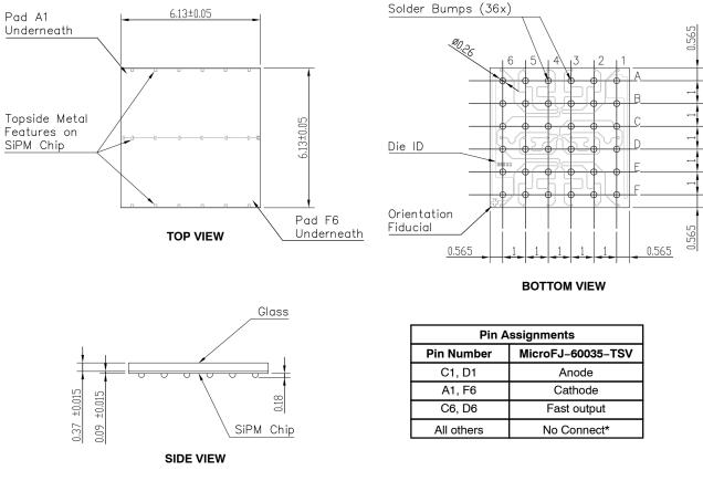
\*The 'No Connect' pins are electrically isolated and should be soldered to a ground (or bias) plane to help with heat dissipation.
