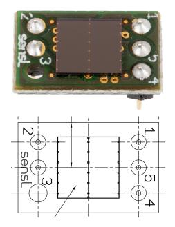
Figure 7. Top View of the SMTPA Board Showing the Pin Numbering
