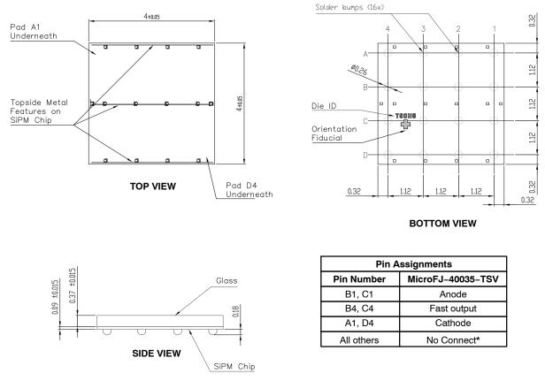
\*The 'No Connect' pins are electrically isolated and should be soldered to a ground (or bias) plane to help with heat dissipation.
