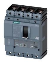
circuit breaker 3VA2 IEC frame 250 breaking capacity class M Icu=55kA @ 415V 4-pole, line protection ETU320, LI, In=250A overload protection Ir=100A...250A short-circuit protection Ii=1.5...10 x In N conductor protection adjustable (OFF, 50%, 100%) nut keeper kit
