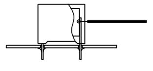
Temperature monitored inside the capacitor.
