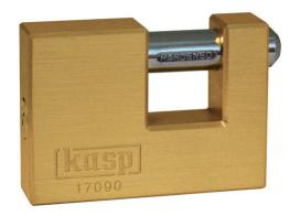
$\sim$  Hardened steel shackle  $\sim$  Solid brass body  $\sim$  5 pin cylinder with anti pick mushroom pins  $\sim$  Extra protection against picking  $\sim$  Paracentric keyway  $\sim$  Supplied with 2 keys  $\sim$  Padlock width: 90 mm  $\sim$  Shackle diameter: 12 mm  $\sim$  Internal shackle height: 18 mm Features & Benefits
