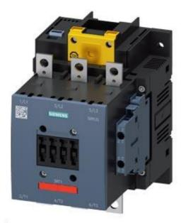
Contactor AC3: 55kW / 400 V 3-pole Size S6 Coil AC 50/60Hz and DC 200...277 V x (0,8...1,1) auxiliary contacts: 2 NO + 2 NC permanently mounted (SUVA) Main: busbar connections coil and auxilliary: screw terminal
