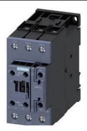
CONTACTOR,AC3:37KW/400V, 1NO+1NC, 48 - 80V AC/DC, WITH VARISTOR, 3-POLE, SIZE S2, SCREW TERMINAL
