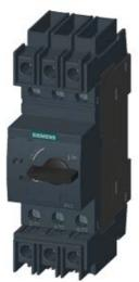
CIRCUIT-BREAKER SZ S00, FOR TRANSFORMER PROTECTION, WITH APPROBATION CIRCUIT-BREAKER UL 489. CSA C22.2 NO.5-02. A-RELEASE 2.5 A, N-RELEASE 52 A, SCREW CONNECTION, STANDARD SW. CAPACITY
