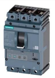
CIRCUIT BREAKER 3VA2 IEC FRAME 100 BREAKING CAPACITY CLASS C ICU=110KA @ 415 V 3POLE, LINE PROTECTION ETU350, LSI, IN=63A OVERLOAD PROTECTION IR=25A ...63A SHORT CIRCUIT PROTECTION ISD=1,5... 10 X IR, II=12 X IN BUSBAR CONNECTION
