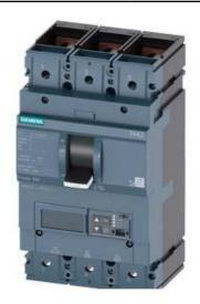
CIRCUIT BREAKER 3VA2 IEC FRAME 630 BREAKING CAPACITY CLASS C ICU=110KA @ 415 V 3-POLE, LINE PROTECTION ETU550, LSI, IN=400A OVERLOAD PROTECTION IR=160A ...400A SHORT CIRCUIT PROTECTION ISD=0,6..10X IN, II=1,5..15X IN NEUTRAL PROTECTION OPTIONAL WITH EXT. CT;UPTO 160% BUSBAR CONNECTION
