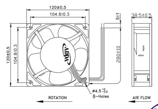
LEAD WIRES : UL 1007, AWG24 , L =  $280\pm10$  mm Red = positive ; Black = negative.
