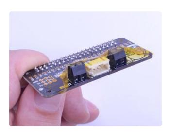
Next we will solder in the 2 3.5mm terminal blocks used to connect speakers to the Speaker Bonnet.
