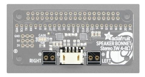
This is the fun part, you get stereo output - one left and one right channel. Each one is Bridge-Tied-Load so do not connect both outputs together to get more volume!
