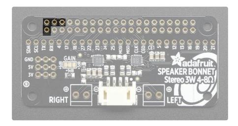
The two amplifier chips use the 3V + 5V + GND power pin at the 'top' of the 2x20 header. If using 3W speakers, you can draw a significant amount of current, over 1.5
