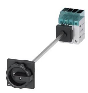
Switch disconnector 3LD3, main switch 3-polig + N, lu 63A operational switch at AC-23 A at 400 V 22,0 kW floor mounting Base mounting with door coupling center-hole 22,5 mm rotary operationg mechanism black  $66 \times 66 \text{ mm}$
