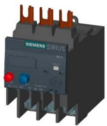
OVERLOAD RELAY 4.5...6.3 A FOR MOTOR PROTECTION SZ S0, CLASS 10, F. MOUNTING ONTO CONTACTOR MAIN CIRCUIT: RING CABLE LUG AUX. CIRCUIT: RING CABLE LUG MANUAL-AUTOMATIC-RESET
