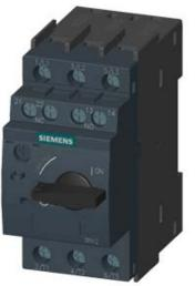
CIRCUIT-BREAKER SZ S00, FOR TRANSFORMER PROT. A-RELEASE 2.8...4A, N-RELEASE 82A, SCREW CONNECTION, STANDARD SW. CAPACITY W. TRANSVERSE AUX. SWITCH 1NO+1NC
