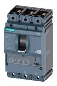
CIRCUIT BREAKER 3VA2 IEC FRAME 100 BREAKING CAPACITY CLASS H ICU=85KA @ 415 V 3POLE, LINE PROTECTION ETU330, LIG, IN=63A OVERLOAD PROTECTION IR=25A ...63A SHORT CIRCUIT PROTECTION II=1,5...12 X IN GROUNDFAULTPROTECTION IG=0,2... 1 X IN, TG=0,1/0,3MS BUSBAR CONNECTION
