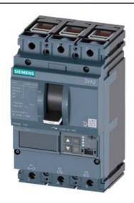
CIRCUIT BREAKER 3VA2 IEC FRAME 160 BREAKING CAPACITY CLASS M ICU=55KA @ 415 V 3POLE, LINE PROTECTION ETU560, LSIG, IN=100A OVERLOAD PROTECTION IR=40A ...100A SHORT CIRCUIT PROTECTION ISD=0,6..10X IN, II=1,5...12X IN NEUTRAL PROTECTION OPTIONAL WITH EXT. CT,UPTO 160% GROUNDFAULT, SWITCHABLE IG=0,2... 1 X IN, TG=0,050,8MS CABLE CONNECTION
