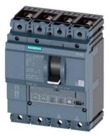
CIRCUIT BREAKER 3VA2 IEC FRAME 250 BREAKING CAPACITY CLASS C ICU=110KA @ 415 V 4POLE, LINE PROTECTION ETU350, LSI, IN=250A OVERLOAD PROTECTION IR=100A ...250A SHORT CIRCUIT PROTECTION ISD=1,5... 10 X IR, II=10 X IN NEUTRAL PROTECTION ADJUSTABLE(OFF,50%,100%) BUSBAR CONNECTION
