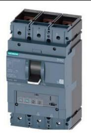
CIRCUIT BREAKER 3VA2 IEC FRAME 400 BREAKING CAPACITY CLASS H ICU=85KA @ 415 V 3-POLE, LINE PROTECTION ETU350, LSI, IN=400A OVERLOAD PROTECTION IR=160A ...400A SHORT CIRCUIT PROTECTION ISD=1,5... 10 X IR, II=10 X IN BUSBAR CONNECTION
