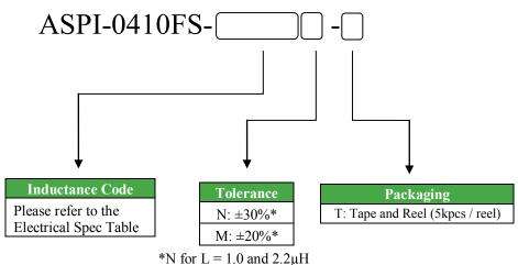
\*N for L = 1.0 and 2.2 $\mu$ H \*M for L = 2.2 ~ 47 $\mu$ H
