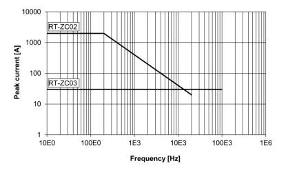
Maximum rated peak input current versus frequency
