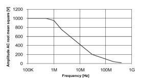
R&S®RT-ZH10/-ZH11 maximum rated sine-wave root mean square voltage versus frequency, CAT I
