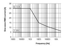
Maximum rated sine-wave root mean square input current versus frequency
