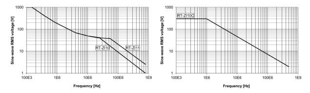
R&S®RT-ZI10(C)/-ZI11 maximum rated sine-wave root mean square voltage between probe tip and probe reference terminal versus frequency (CAT III)
