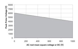
R&S®RT-ZH10/-ZH11 maximum root mean square voltage versus peak pulse voltage, CAT I
