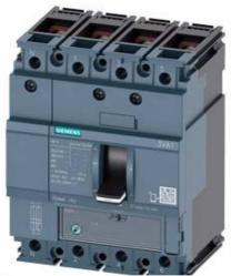
CIRCUIT BREAKER 3VA1 IEC FRAME 160 BREAKING CAPACITY CLASS N ICU=25KA @ 415 V 4-POLE, LINE PROTECTION TM220, ATFM, IN=125A OVERLOAD PROTECTION IR=87,5A ...125A SHORT CIRCUIT PROTECTION II=10 X IN NEUTRAL UNPROTECTED BUSBAR CONNECTION
