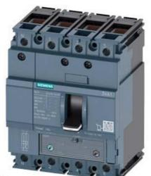
CIRCUIT BREAKER 3VA1 IEC FRAME 160 BREAKING CAPACITY CLASS H ICU=70KA @ 415 V 4-POLE, LINE PROTECTION TM240, ATAM, IN=20A OVERLOAD PROTECTION IR=14A ...20A SHORT CIRCUIT PROTECTION II=5...10 X IN NEUTRAL UNPROTECTED CABLE CONNECTION
