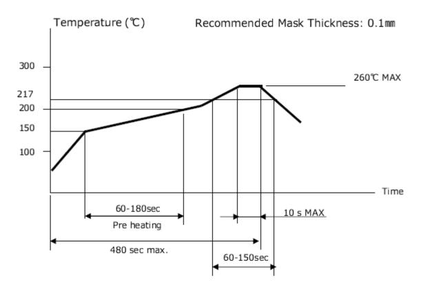
Temperature on the surface of PWB
