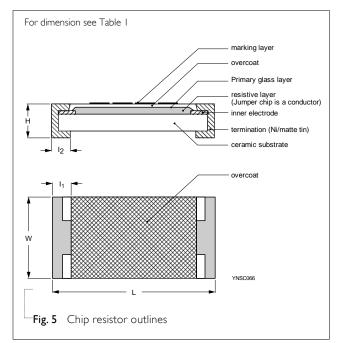
**4** 10 Chip Resistor Surface Mount RV series 0603/0805/1206/2010/2512 (RoHS Compliant)
