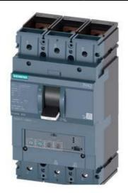
CIRCUIT BREAKER 3VA2 IEC FRAME 400 BREAKING CAPACITY CLASS M ICU=55KA @ 415 V 3-POLE, LINE PROTECTION ETU330, LIG, IN=400A OVERLOAD PROTECTION IR=160A ...400A SHORT CIRCUIT PROTECTION II=1,5...10 X IN GROUND-FAULT-PROTECTION IG=0,2... 1 X IN, TG=0,1/0,3MS BUSBAR CONNECTION
