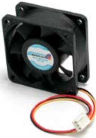
The StarTech.com FAN6X25TX3H is a 5000 RPM, 6 x 2.5cm fan designed to prevent computer systems from overheating, thereby increasing efficiency and stability. Featuring a TX3 end and a built-in tachometer that sends RPM signals to your motherboard, the FAN6X25TX3H is a high-performance way to avoid overheating and system failure.
