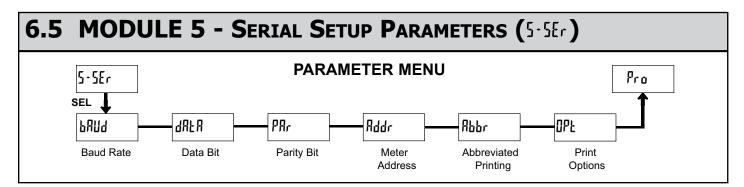
The Serial Setup Parameters are only active when one of the optional serial communications/programming cards is installed in the meter. Refer to the CUB5COM bulletin for details and setup for the CUB5 RS232 or RS485 serial communications. Refer to the CUB5USB bulletin for details on the CUB5 USB programming and programming requirements.
