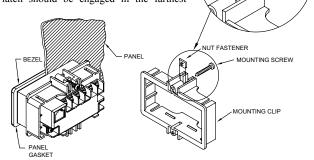
forward slot possible. To achieve a proper seal, tighten the latch screws evenly until the unit is snug in the panel (Torque to approx. 28 to 36 in-oz [0.202 to 0.26 N-m]). Do not over-tighten the screws.
