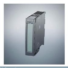
SIMATIC S7-1500, digital output module DQ 16x 230V AC/2A ST; relay 16 channels in groups of 2; 4 A per group; switching cycle counter for integrated relay, diagnostics; substitute value: the module supports the safety-oriented shutdown of load groups up to SIL1 according to EN IEC 62061:2021 and Category 2 / PL c according to EN ISO 13849-1:2015. front connector (screw terminals or push-in) to be ordered separately
