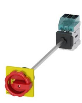
Switch disconnector 3LD3, main switch 3-polig, lu 25A operational switch at AC-23 A at 400 V 9,0 kW floor mounting Base mounting with door coupling center-hole 22,5 mm rotary operationg mechanism red/yellow 66 x66 mm
