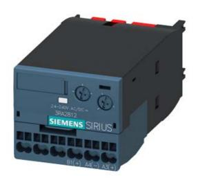
SOLID-STATE TIME RELAY OFF-DELAY WITH AUXILIARY VOLTAGE AND SEMICONDUCTOR OUTPUT 24...240V AC/DC TIME RANGE 0.05...100S FOR SNAPPING ONTO THE FRONT; FOR 3RT2 CONTACTORS S00/S0 SPRING-TYPE TERMINALS INTEGRATED VARISTOR FOR DAMPING CONTACTOR COILS
