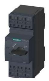
CIRCUIT-BREAKER SZ S0, FOR MOTOR PROTECTION, CLASS 10, A-REL. 5.5...8A, N-REL. 104A SPRING-L. CONNECTION, STANDARD SW. CAPACITY
